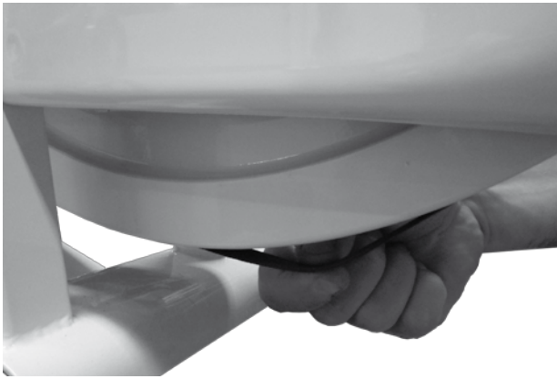
Fig: Control loose brake belt
